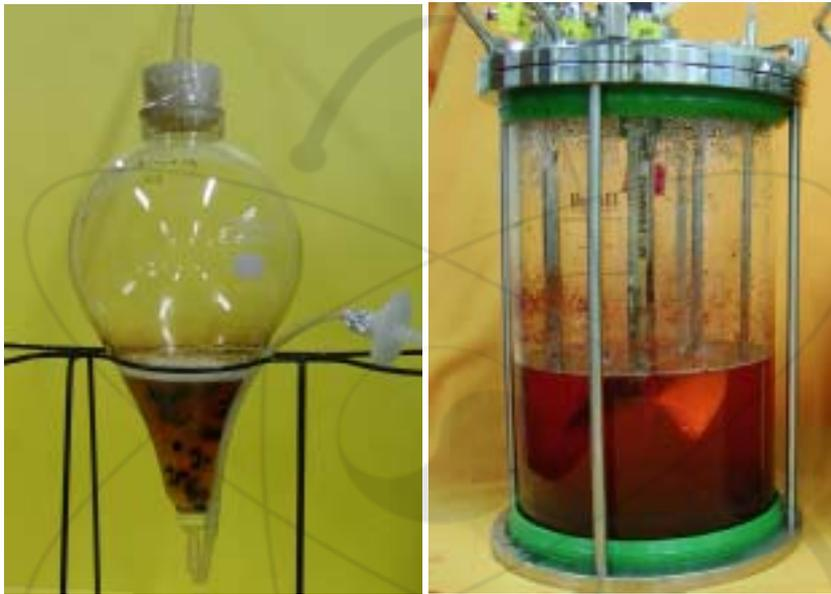
Figure 2. Bioreactor(left, 5 L; right, 7 L vessel) for cell suspension culture of *L. erythrorhizon*.
