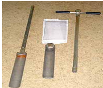
Figure 2 Equipment for sediment sampling
