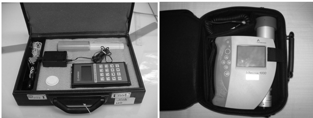
Figure 1. Left: RKG-AT1320 thyroid monitor: NaI(Tl) detector, control unit, charger, ^{137}\text{Cs} control source and cables. Right: InSpector 1000 thyroid monitor: In addition to spectrum acquisition mode the Inspector monitor can be used in dose rate mode or in nuclide identification mode.
