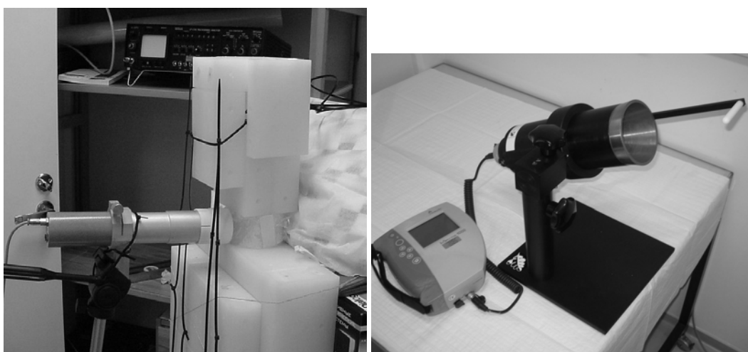
Figure 2. Left: RKG-AT1320 thyroid monitor in a 5 mm lead collimator and an adult phantom in measurement distance of 7 cm. Right: InSpector 1000 thyroid monitor in a table-top lead shield.
