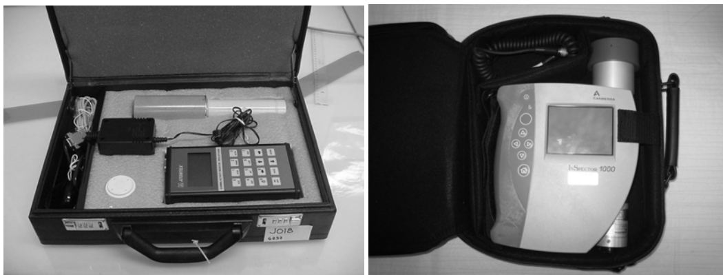
Figure 1. Left: RKG-AT1320 thyroid monitor: NaI(Tl) detector, control unit, charger, ^{137}\text{Cs} control source and cables. Right: InSpector 1000 thyroid monitor: In addition to spectrum acquisition mode the Inspector monitor can be used in dose rate mode or in nuclide identification mode.
