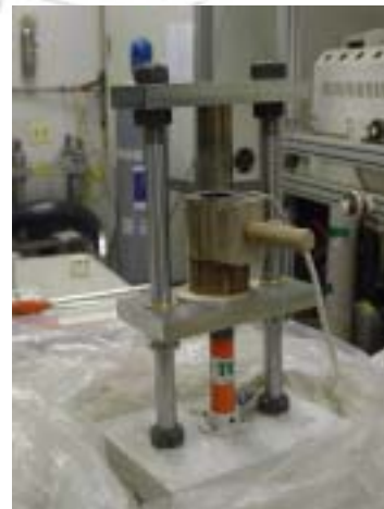
Fig. 7. Hot-forging system for stacking of slurry infiltrated fabrics.
