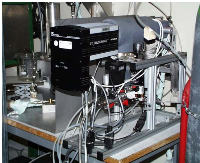
Figure 9: Thermogravimetric furnace and mass spectrometer used for the MOZART programme
