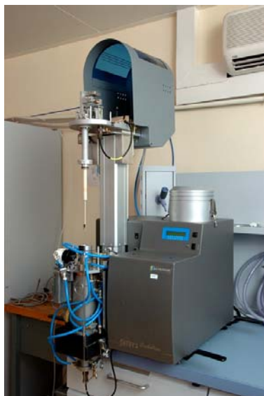
Figure 9: Thermogravimetric furnace and mass spectrometer used for the MOZART programme
