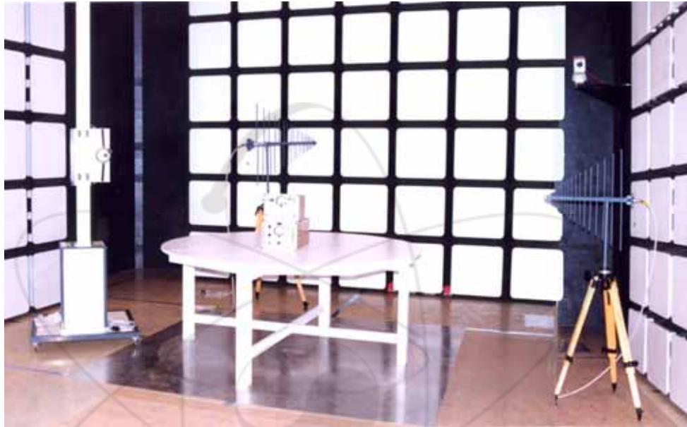
Fig. 3. Screened anechoic test chamber
