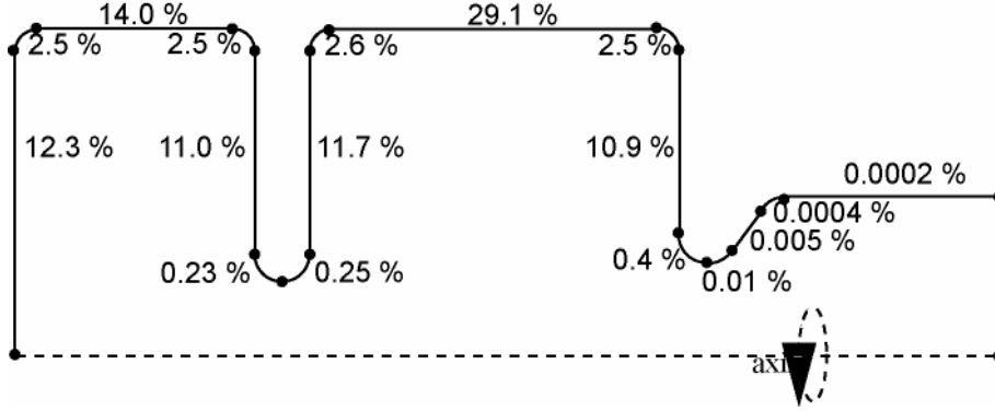
Figure 10: Relative power entries at specified wall segments around the rf-gun internal boundary as calculated with SUPERFISH.
