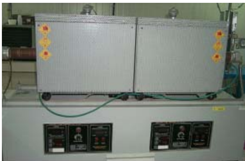
Figure 23. Photograph of two-zone furnace.
