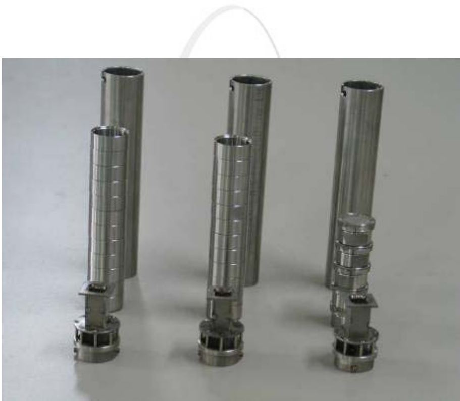
Figure 2. First filter units manufactured by KAERI.
