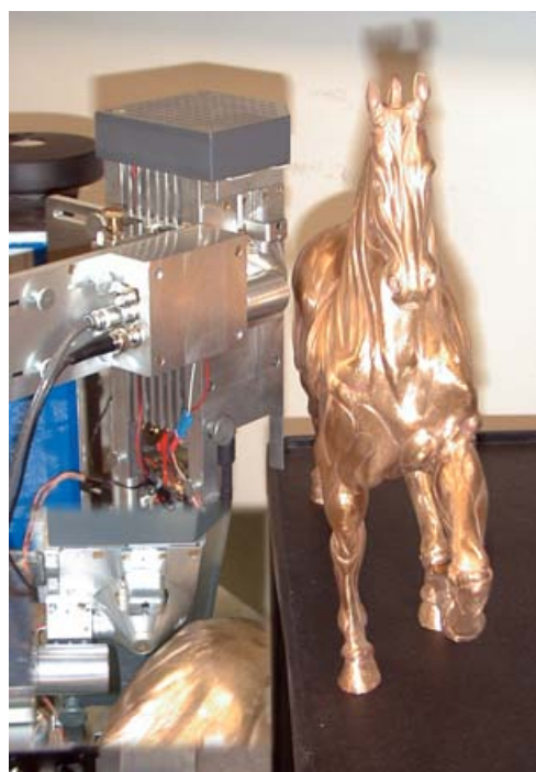
Fig. 1. The portable XRF spectrometer performing the analysis of a horse statue. In the left lower corner a close-up of the excitation geometry is shown.
