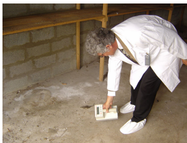
Figure 1: Measurement of the floor contamination on the on site inspection of the SNSA at the IJS.
