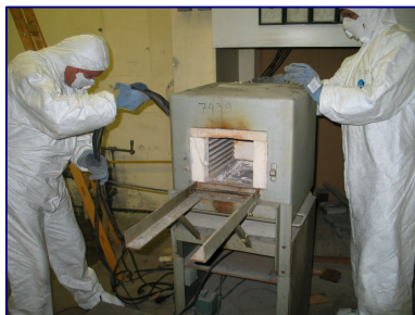
Figure 3: Decontamination of contaminated oven which was used in the past in the research of uranium compound at the IJS. The picture was provided by the IJS.
