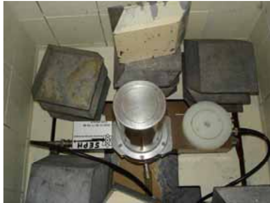
Fig. 11: The detector with its Pb shielding
