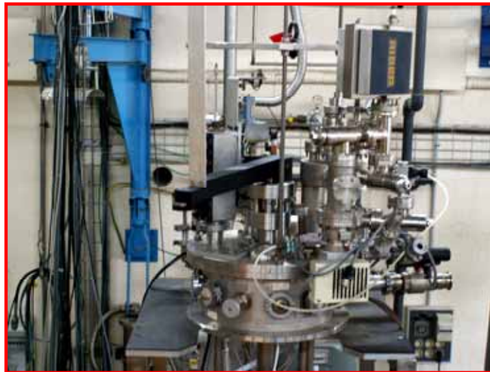
Fig. 6: Photograph of the upper part of the insert ready for cryogenic test
