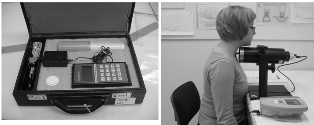
Figure 4. Left: RKG-AT1320 thyroid monitor: NaI(Tl) detector, control unit, charger, ^{137}\text{Cs} control source and cables. Right: InSpector 1000 thyroid monitor in a table-top lead shield.
