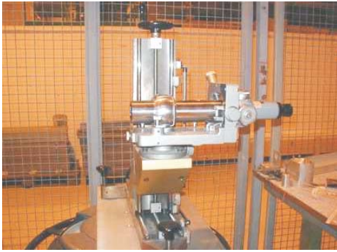
Fig. XII. Socket for laboratory metrology and specific gauge (CERN TS-SU-EM library)
