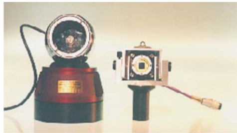
Fig. VIII. The fiducial reference point and the measurement station and various types of brackets (CERN TS-SU-EM library)
