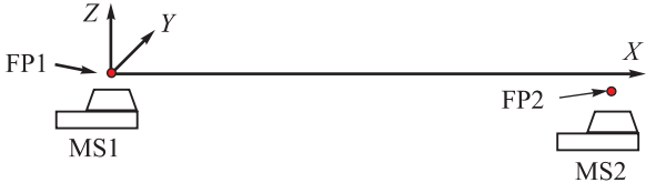
Fig. III. A conventional reference frame of a local XYZ coordinate system
