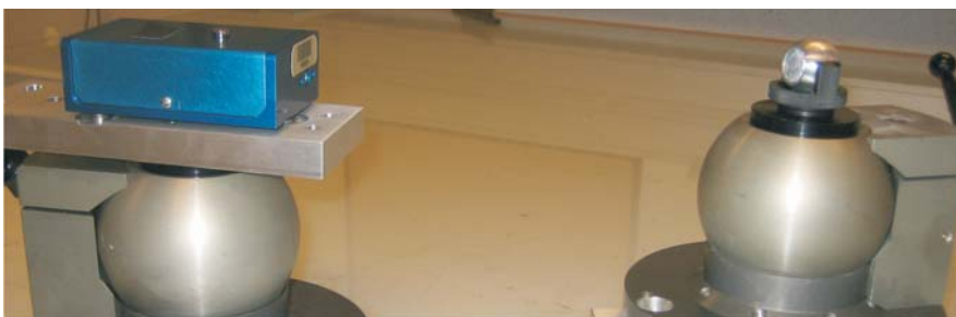
Fig. XI. Specific socket adaptations for various types of measures (CERN TS-SU-EM library)
