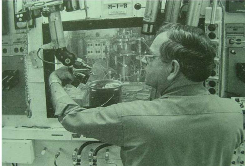
Figure 2. Remote Loading of Radioactive Waste into a 16.5 L Can, Hot Cell M-1.
