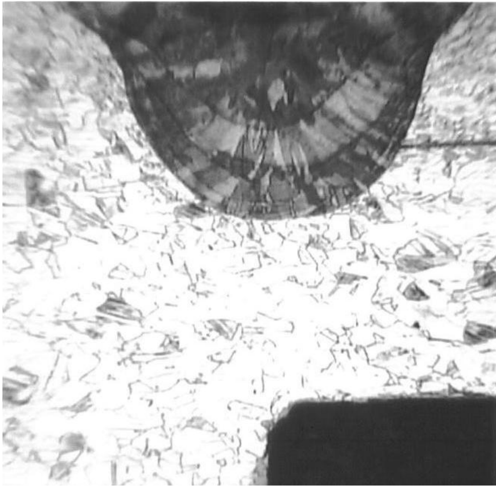
Figure10 Microstructure of the weld
