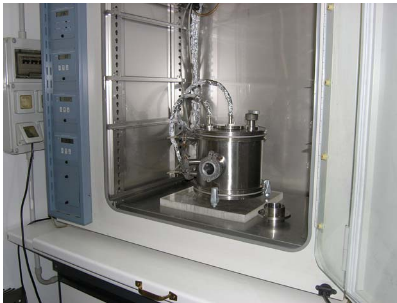
Figure 3. The alpha-irradiator placed into a standard CO 2 incubator
