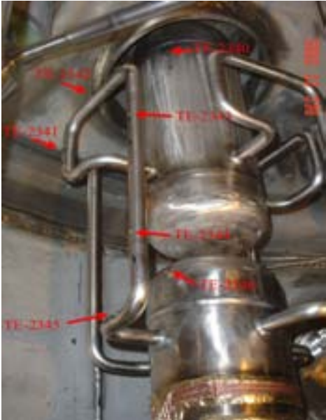
FIG. 8. Hydrogen pressurizer and temperature element location map.
