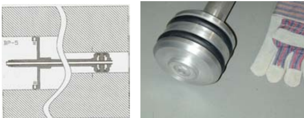
FIG. 5. Beam port plug showing expanding seal area.
