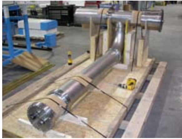
FIG. 19. Test heater assembly.
