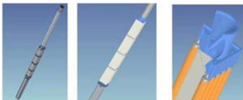
FIG. 3. Spatial views of the new control rod.
