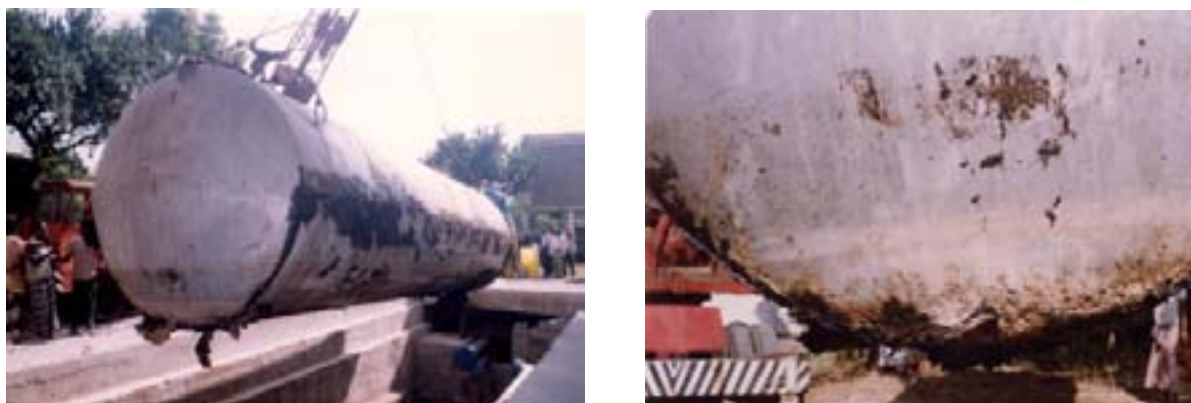
FIG. 1. Removal of the damaged ^{16}\text{N} decay tank and marks of corrosion pitting on its surface.
