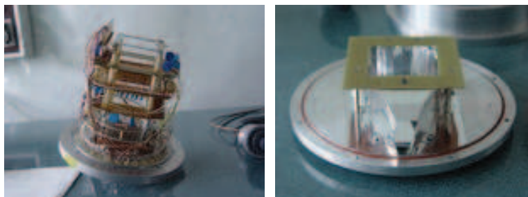
Figure 1: Ionization part (left side) and the scintillation part (right side) of the SID detector.
