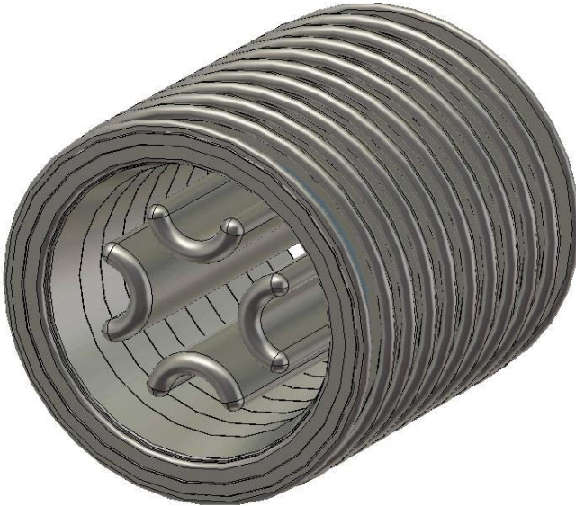
Figure 5: View of an entire tube section showing all four quadrupole electrodes.
