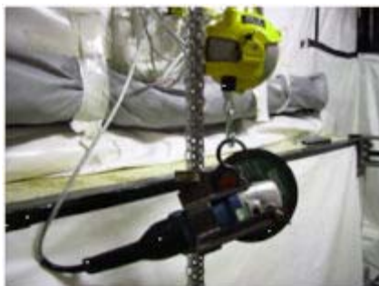
Figure 14: Remote grinding operations in shielded containment
