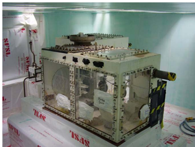
Figure 5: Glove-box prepared for decommissioning
