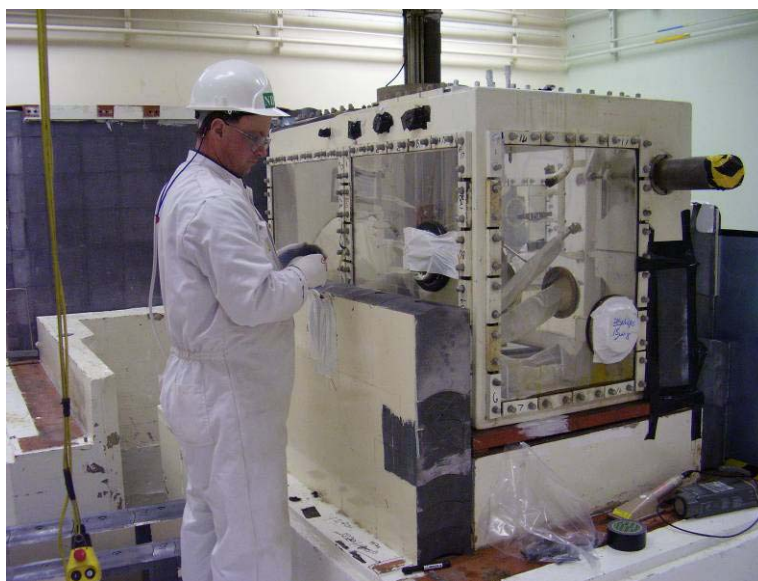
Figure 2: A glove-box with some of its shielding removed
