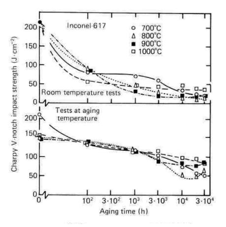
Heat to heat variation significant Minimum Values: tests at RT Heat effected zone data very low: ~ 10 J
