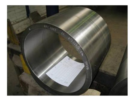
Section of a HR-pipe with a wall thickness of ca. 30mm
