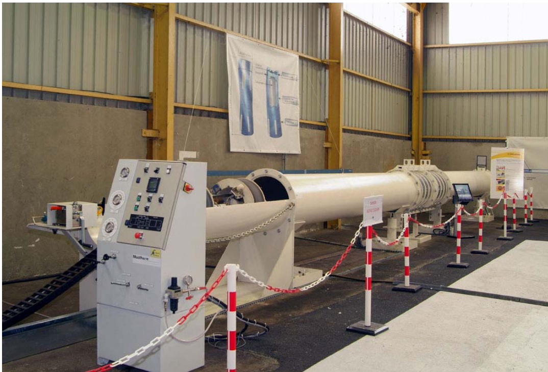
Figure 11: General view of the P1 Test Bench, also showing the Prototype Pushing Robot and the Control Panel
