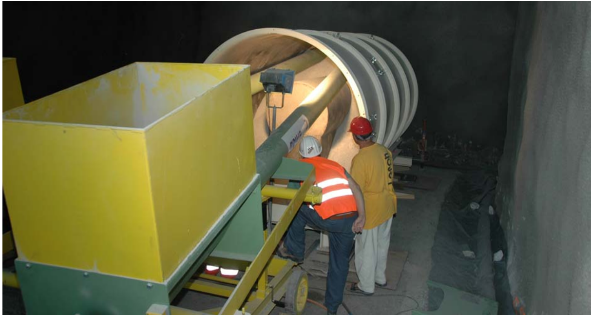
Figure 10: Experiment testing the emplacement of bentonite granulate
