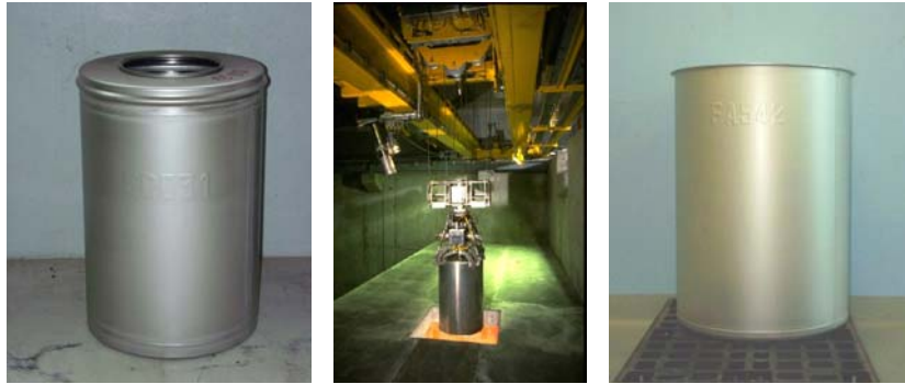
Figure 2: ILW-LL Stainless steel drums
