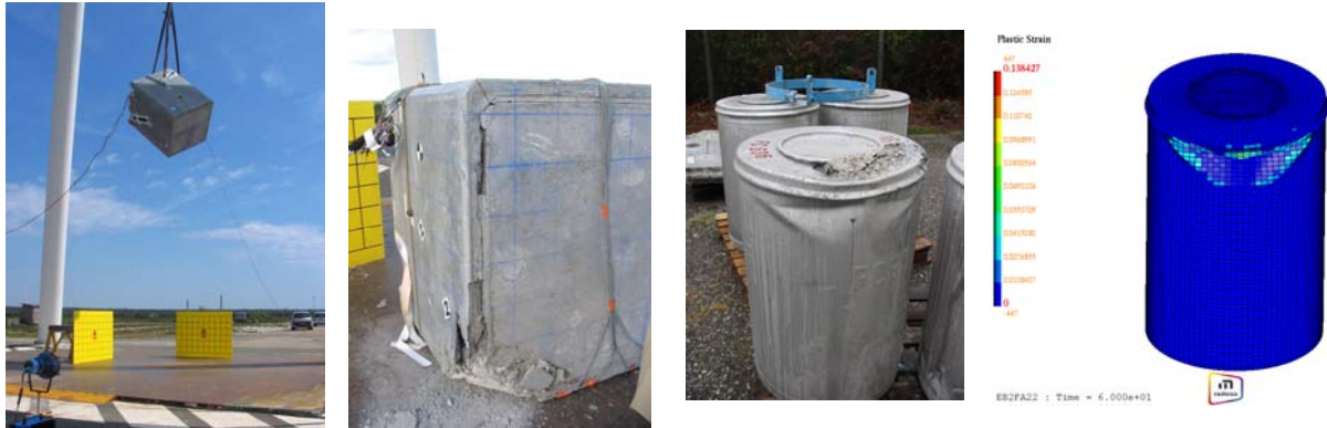
Figure 9: Corner drop test on disposal package and bitumen drums – Comparison with simulation
