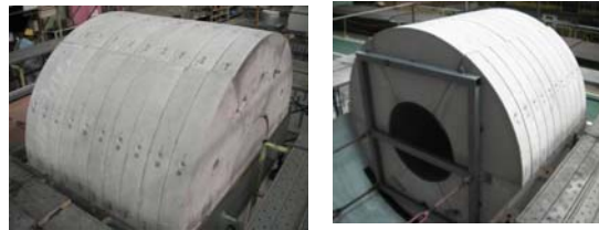
Figure 12: Completed EBS assemble
