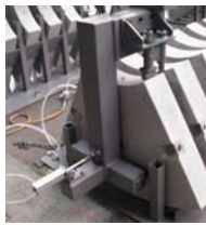
Figure 11: Hoisting device for blocks
