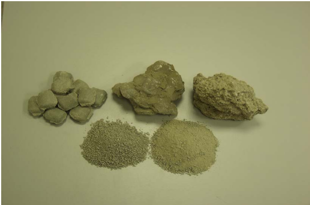
Figure 1: Bentonite compacts (briquettes, granulates) and binary Bentonite mixture after dismantling.
