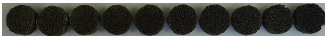
Fig. 16. Photograph of fly ash filters after trapping cesium and molybdenum under a vacuum of 0.13 torr.
