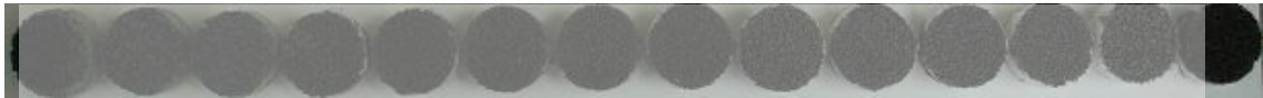
Fig. 14. Photograph of fly ash filters after trapping cesium under a vacuum of 76 torr.
