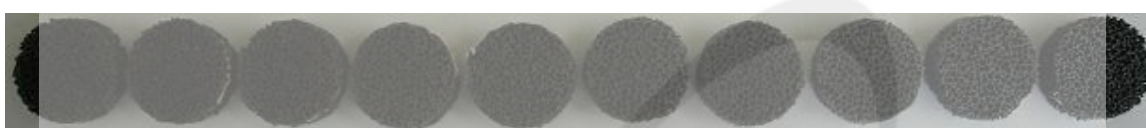
Fig. 11. Photograph of fly ash filters after trapping cesium under a vacuum of 0.2 torr.
