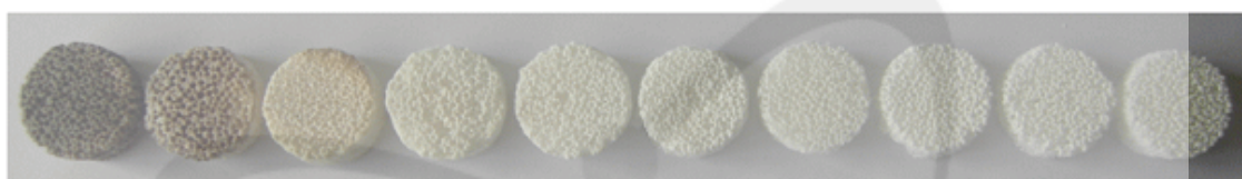
Fig. 42. Photograph of Ca-II filters after trapping molybdenum, rhenium, antimony, and tellurium under a vacuum of 7.6 torr.
