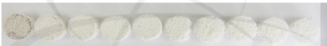
Fig.34. Photograph of Ca-II filters after trapping rhenium under a vacuum of 76 torr.
