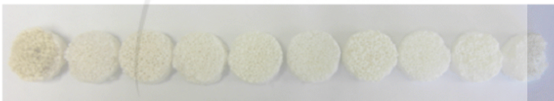
Fig. 37. Photograph of Ca-II filters after trapping antimony under a vacuum of 7.6 torr.
