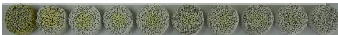
Fig. 24. Photograph of Ca-I filters after trapping rhenium under a vacuum of 76 torr.
