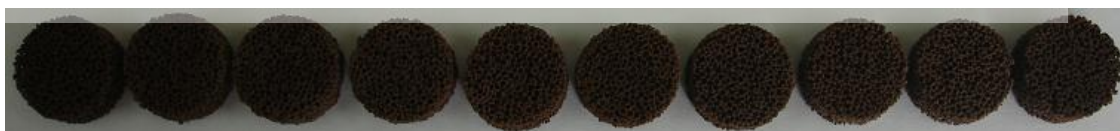
Fig. 7. Photograph of fly ash filters after trapping gaseous cesium under a vacuum of 2.7 torr.
