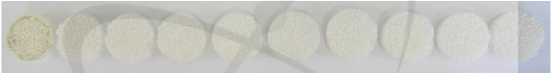
Fig. 40. Photograph of Ca-II filters after trapping tellurium.
