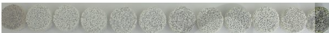
Fig. 20. Photograph of Ca-I filters after trapping ruthenium under a vacuum of 7.6 torr.
