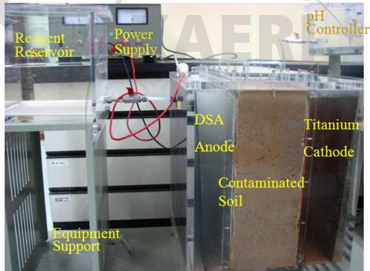
Fig. 19. Manufactured electro-chemical flushing equipment
