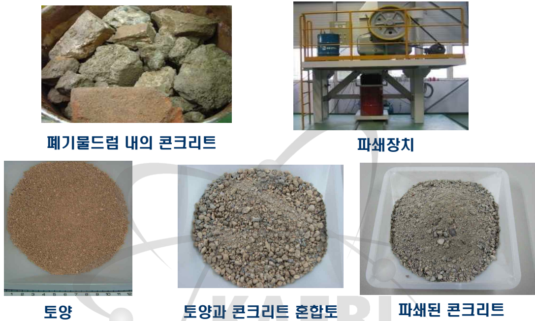
Fig. 5. The crushing and mixture of concrete
