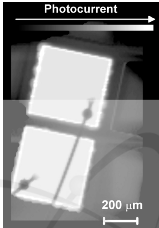
Figure 12. X-ray photocurrent maps of two 4H-SiC Schottky diodes ( 400 \times 400 \mu\text{m}^2 ).
