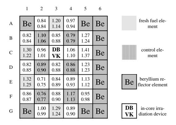
Figure 2: mean radial power peaking form factors at balanced rod position for the 1<sup>st</sup> LEU standard core at BOC (first value) and EOC (second value)
