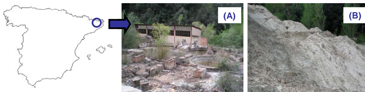
Fig. 3. Location of the studied mining area (North-East of Spain) and impact of abandoned mining activities: (A) ore concentrate tanks, (B) accumulation of mining wastes.
