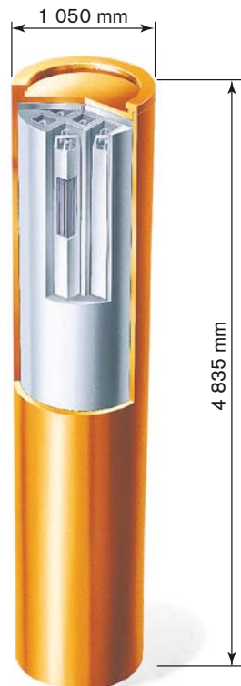
Figure 1-1. Canister for final disposal of spent nuclear fuel.
