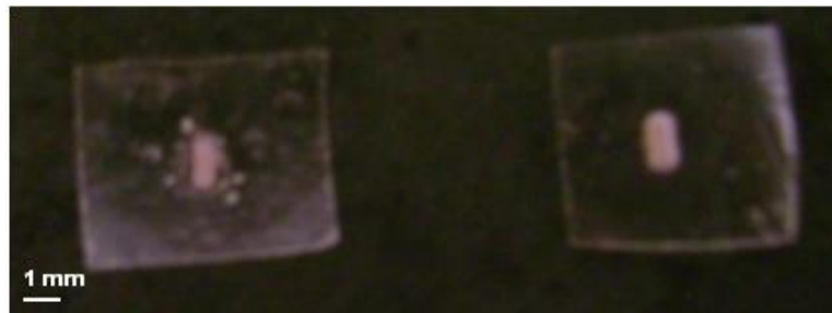
Figure 1 - Bioglass seeds of [Si: Ca: Ho] and [Si: Ca: Ho: Zr], encapsulated in membranes of polyvinyl alcohol.
