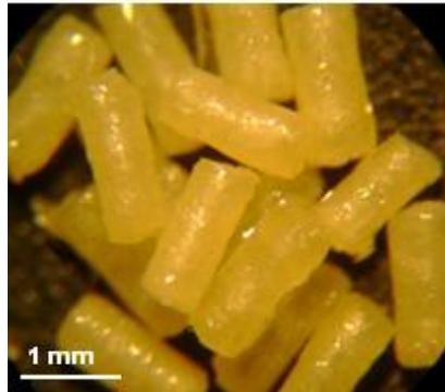
Figure 2 - Bioglass seeds of [Si: Ca: Ho: Zr] encapsulated with acrylate resin obtained in stereoscopic 80X.
