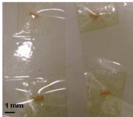
Figure 4 – Bioglass seeds of [Si: Ca: Ho] and [Si: Ca: Ho: Zr] mounted on acrylic plaque.
