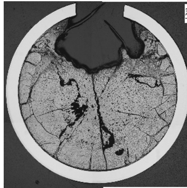
Standard \text{UO}_2 pellet after inreactor washout test
