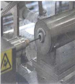
Drilling of hole in fuel rod for attaching high temperature thermocouple.
