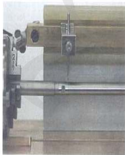
TIG-welding of instrumented end-plug onto a fuel rod.
