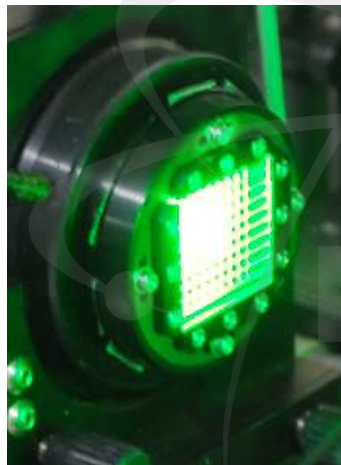
Fig. 3-9. Photo of a beam homogenizer (left) and cylinder type lens of beam homogenizer (right).
