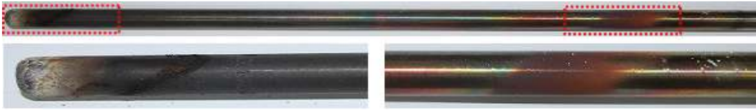
Fig. 2-6. Zircaloy surface covered with metal oxide deposits: test solution: 20 ppm Fe, 5 ppm Ni, 5 ppm Zn, 0.5 ppm Cr and 0.5 ppm Si (320°C, 12.5 MPa, for 40 h).
