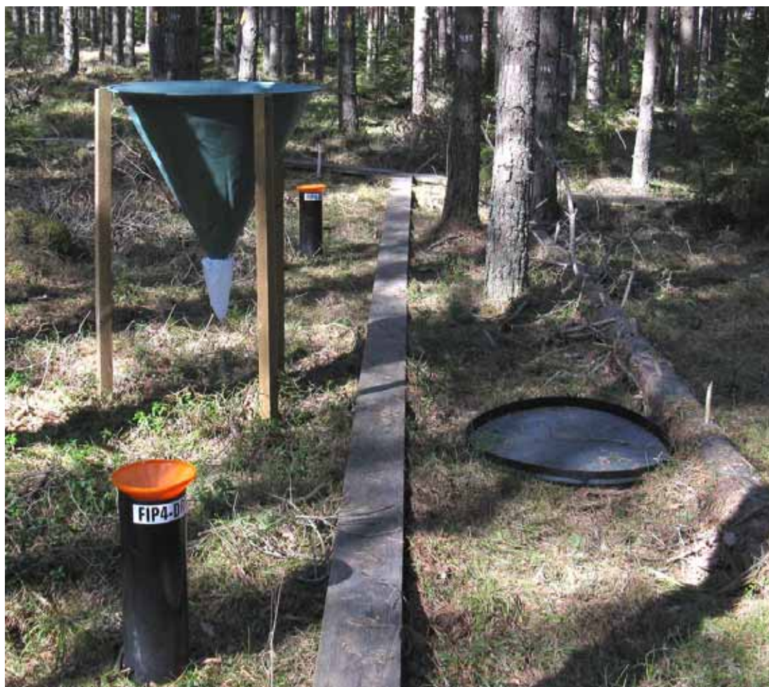
Figure 6. Litterfall traps on an FIP plot. Green funnel type litterfall trap used in ICP Forests programme (UN/ECE 2004a) and new "branch trap" (circle on the ground on the right side) developed to collect branch litter. (Photo: L.Aro/ Metla).
