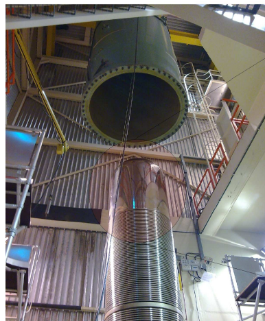
7 MeV VdG Column filled with up to 15 bars of Nitrogen
