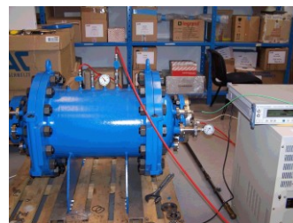
3.a) Pressure test tank
