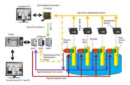
Figure 8: Detail Design of ACSCR with Complete Setup
