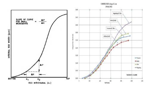
Figure 3: Integral Control Rod Worth
