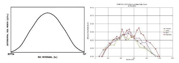
Figure 4: Differential Control Rod Worth
