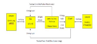
Figure 6: Conceptual Design for ACSCR
