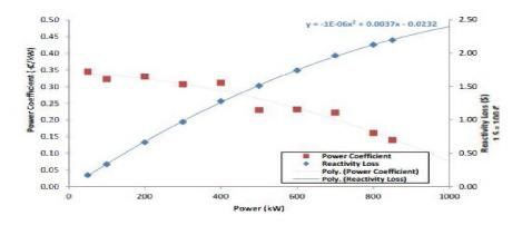
Figure 5: Power coefficient of reactivity and reactivity loss versus reactor power level
