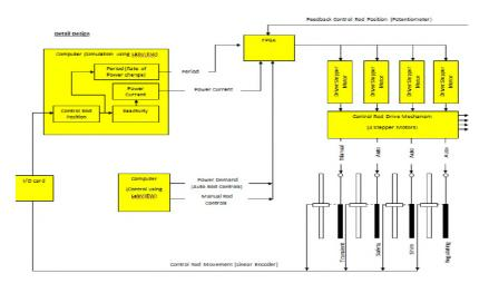
Figure 7: Detail Design for ACSCR
