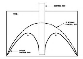
Figure 2: Effect of Control Rod on Radial Flux Distribution
