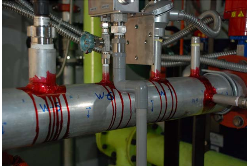
Figure 4: Dye penetrant application
