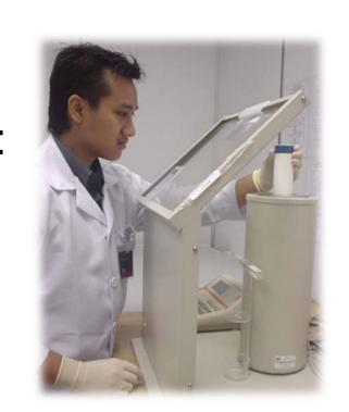
Linearity test could be performed using either decay method or shield method.
