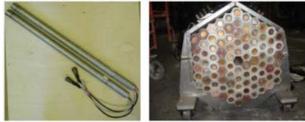
Fig. 1. The ^3\text{He} tubes (left). The schematic view of TETRA neutron detector before the update (right). See the text for details
