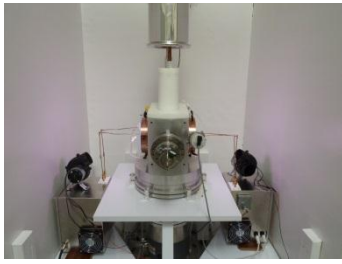
FIG. 4. The UC Berkeley neutron generator expected to be running in the summer of 2013.
