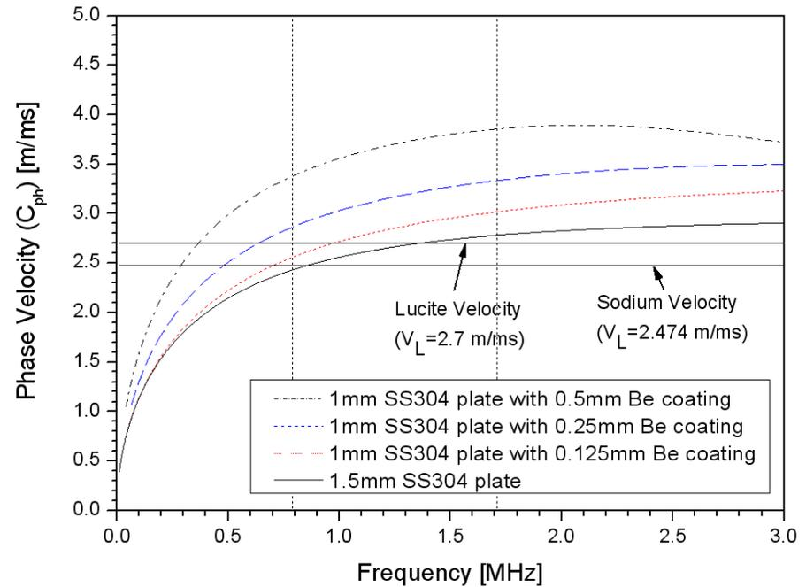
**Phase Velocity of Be Coating Plate**
