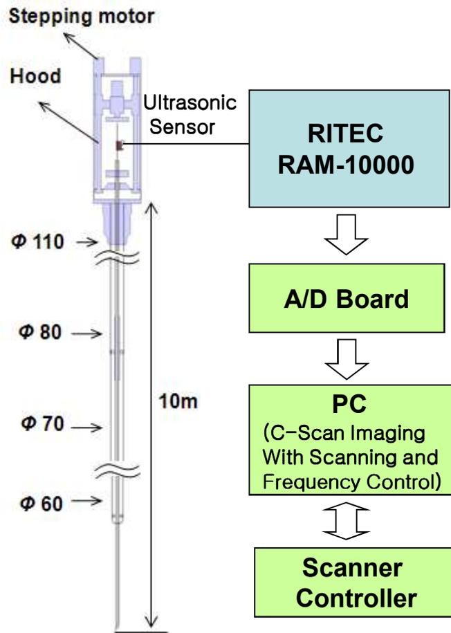
C-Scan Test of 10 m Single Waveguide Sensor Module
