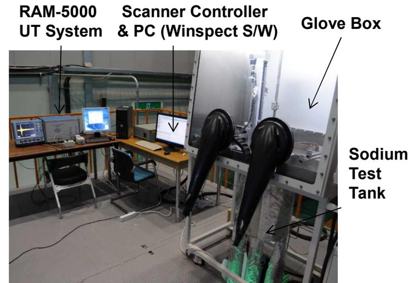
Glove Box with Sodium Test Tank And UT System
