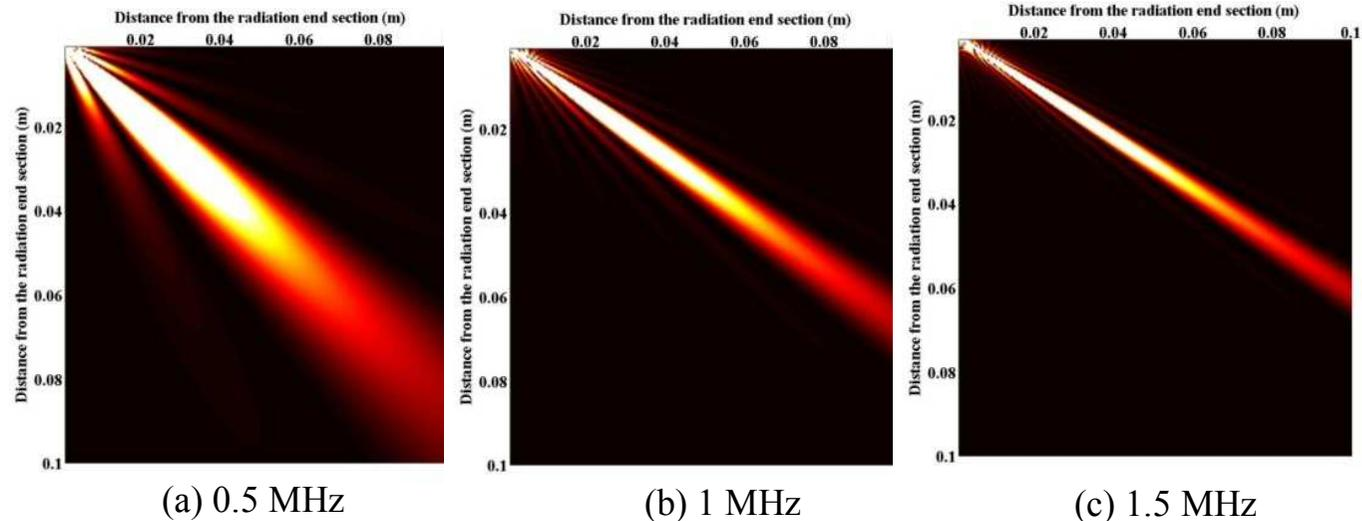
**Radiation Beam Profiles (in Water)**
