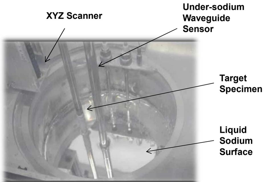
C-Scan Imaging Test in Sodium
