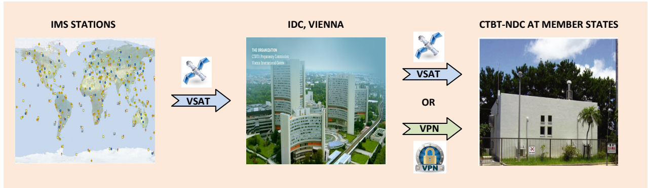
Figure 1. Transmission of the monitoring data from IMS Stations to CTBT-NDC
