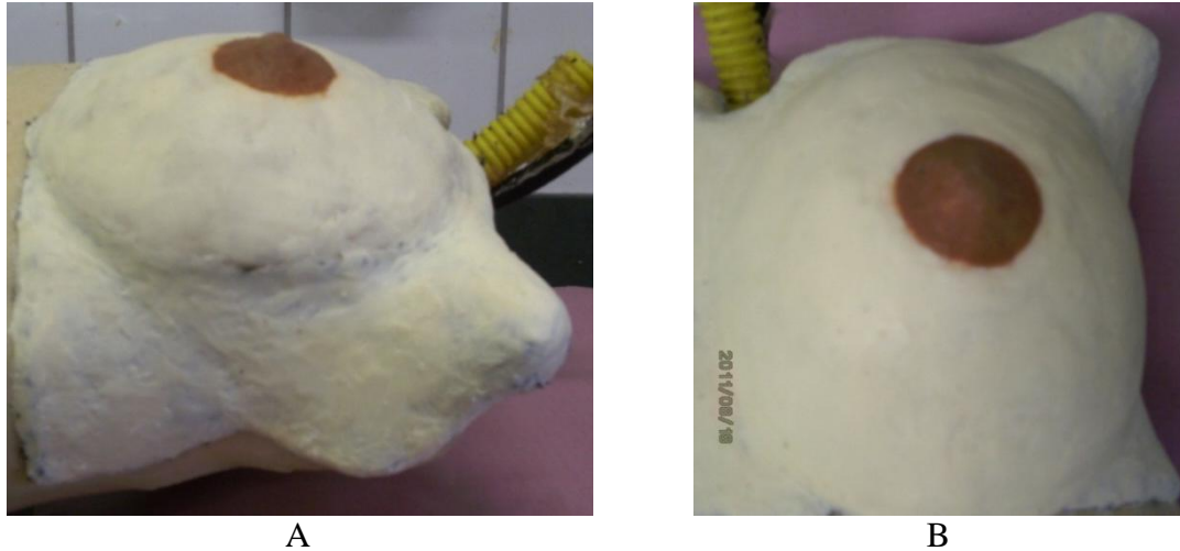
Figure 4: anthropomorphic and anthropometric breast phantom (A) side view (B) upper view.
