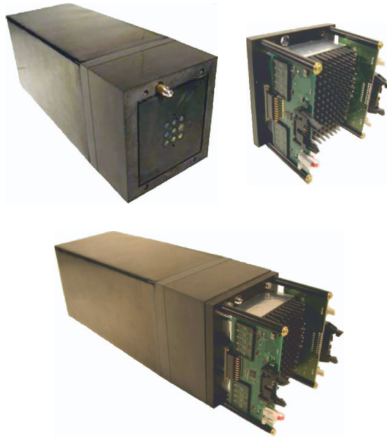
Fig. 2. View of the Shashlyk calorimeter module and components
