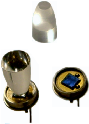
Fig. 7. View of the MAPD with and without the Winston cone
