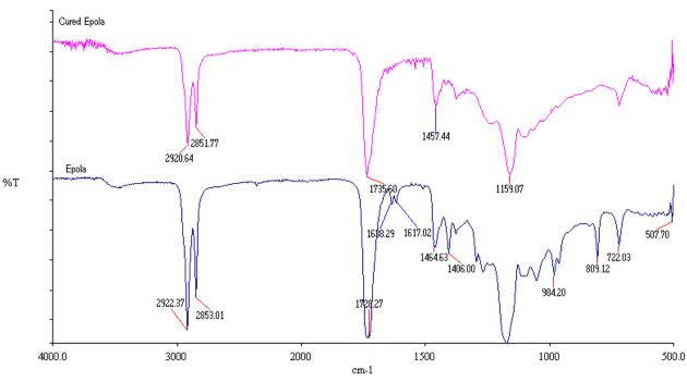
Figure 3: FTIR spectra of EPOLA and cured EPOLA
