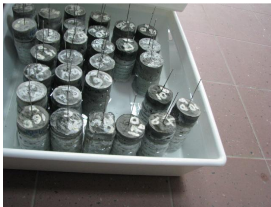
Figure 1 Samples immersed in NaCl 3.5% solution
